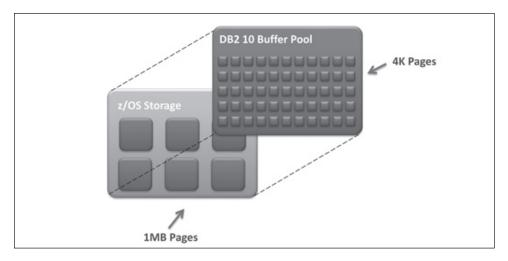
Figure 11: Buffer pool using 1MB z/OS page size
