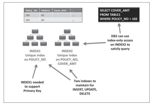
Figure 8: Multiple indexes to support index-only access
